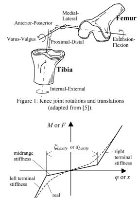
Figure 2: Elastic joint moment or force as function of rotational or translational displacement, respectively.
